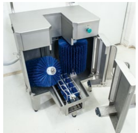
Simple opening for cleaning purposes
